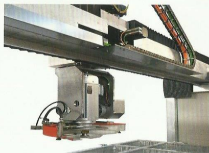
Disco inclinato a 90°. Disc inclined at 90°.
